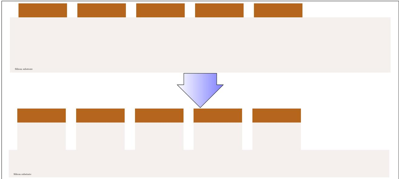
**Figure 3:** Trench etching
