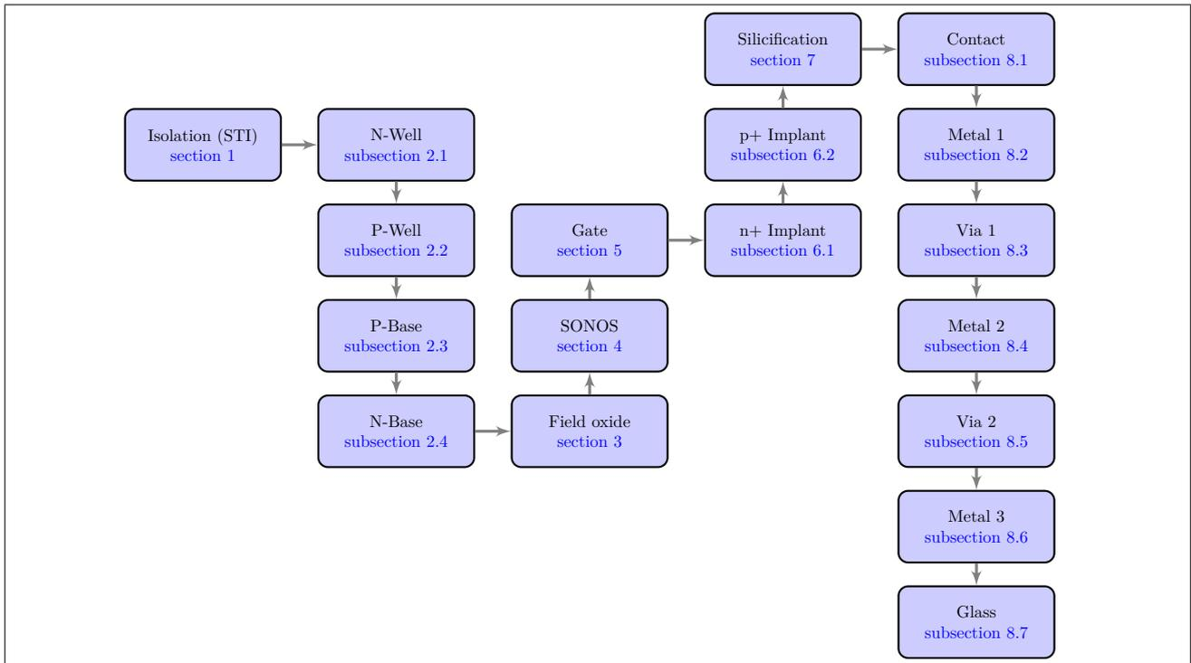
**Figure 1:** Frontend and backend process flow
