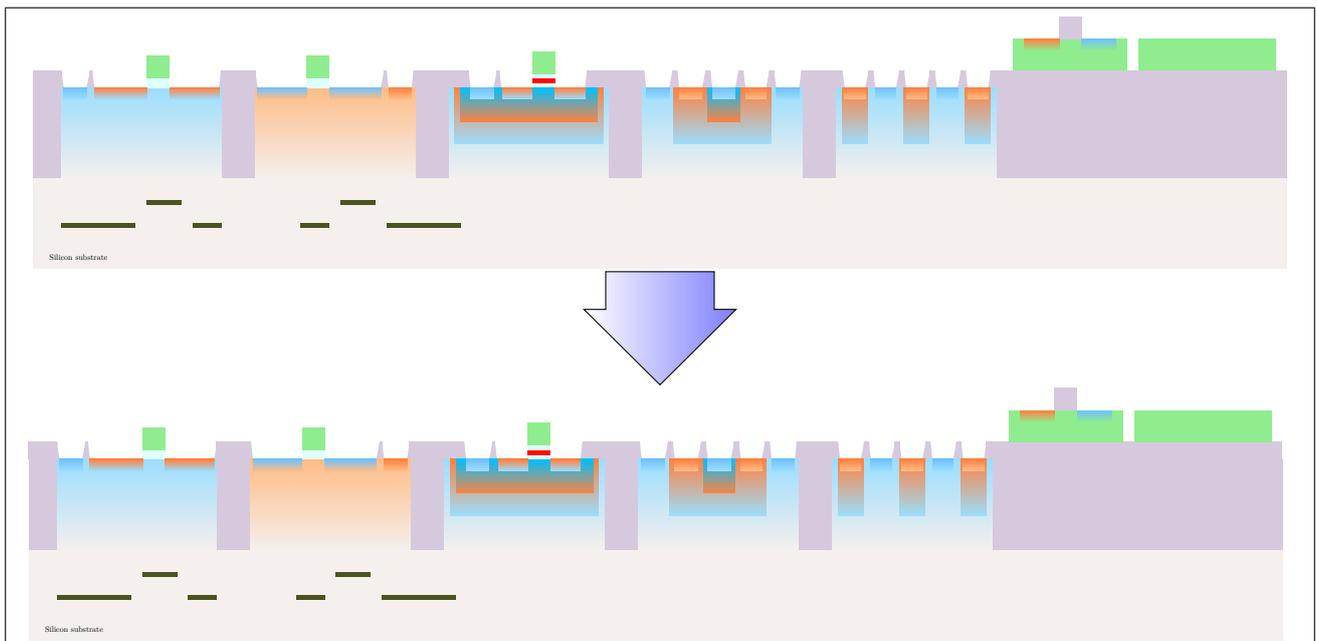
**Figure 32:** Titanium etch
