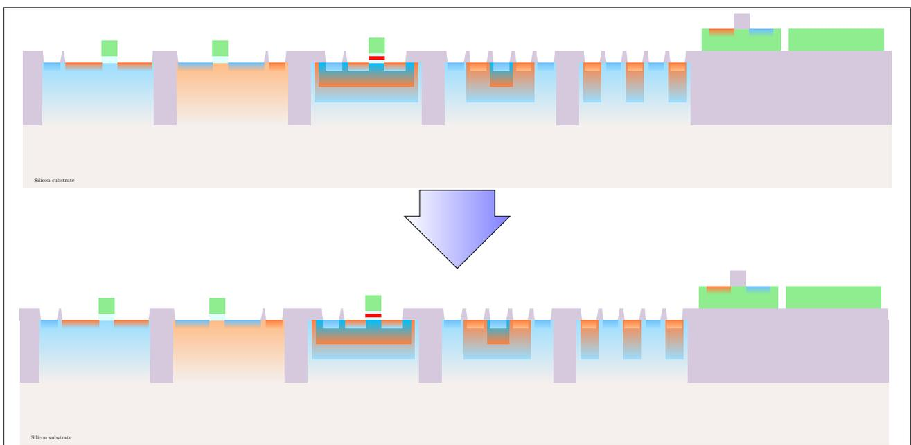
**Figure 30:** Titanium deposition
